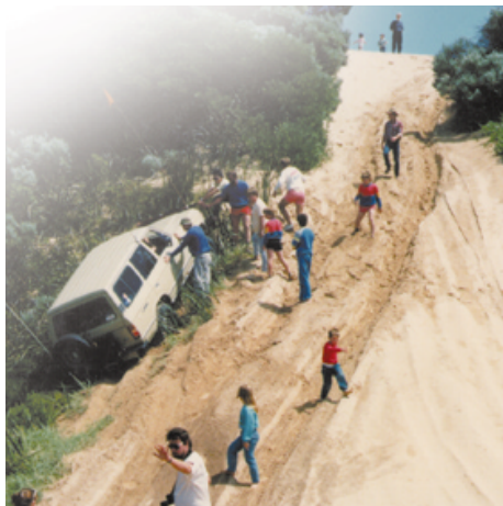
The Landcruiser pictured bounced right off the track due to too much speed with too little suspension travel and suppleness. Look closely at the tracks.
