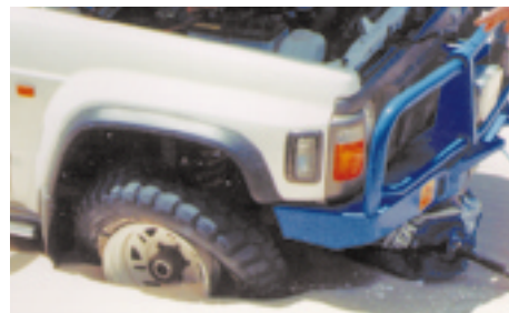
Tyre off bead in sand
