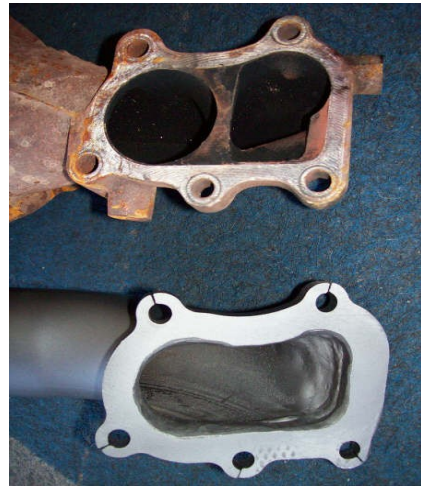
Dump pipe flange
