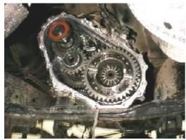
Unbolt rear case, remove gears
